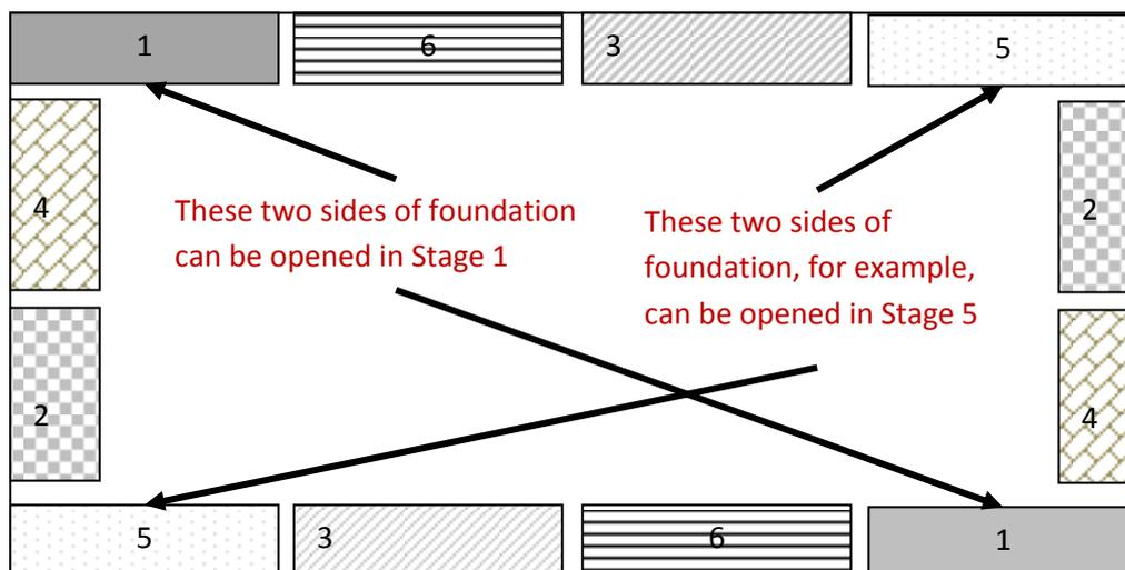
Figure 4-1 Schematic diagram showing stage-wise retrofitting of foundation of load-bearing masonry walls
