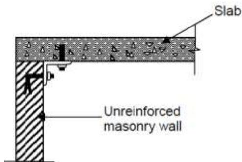
Figure 3-6 Anchorage of slab/floor with masonry wall
