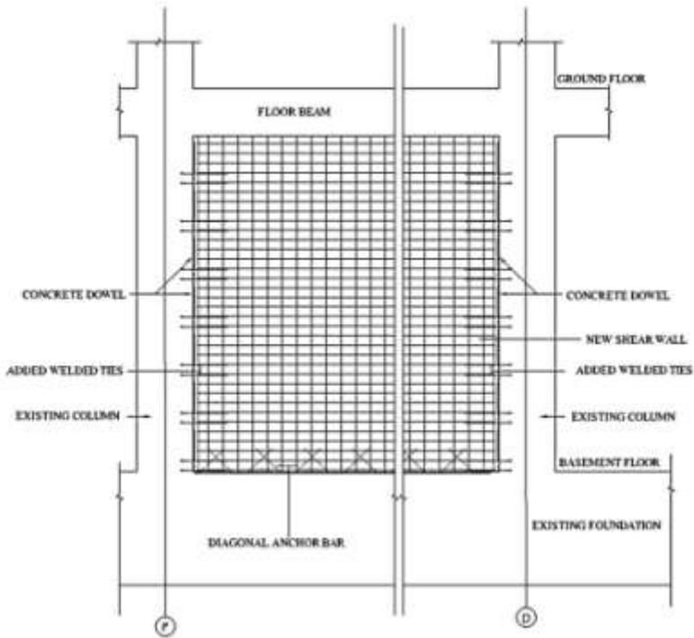
Figure 3-2 Introduction of a new shear wall
